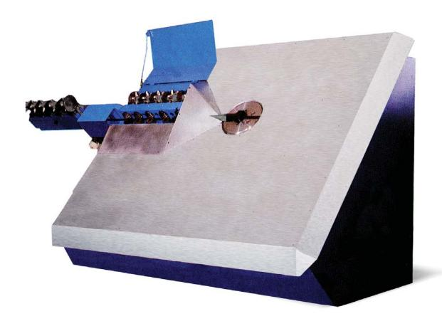
DIAS 16 is an advanced CNC Programmable Two - Axis Straightening, Bending & Cutting machine, designed to product structural stirrups and others (from reinforced rod bars) for concrete reinforcing applications.
